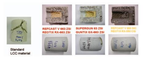
Figure 1. Alkali bursting test (5 h at 1100 °C with K<sub>2</sub>CO<sub>3</sub>)
